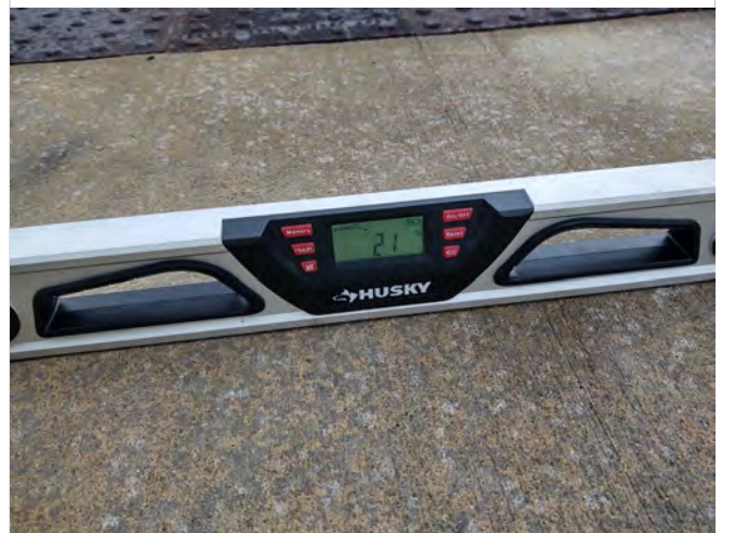
Photo AMN4 – Cross slope of curb ramp at 2.1%.
