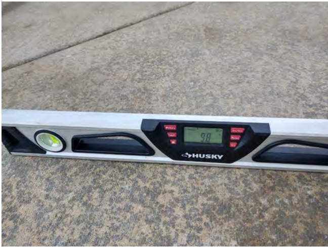
Photo AMN3 – Side running slope on other side of curb ramp at 9.8%.
