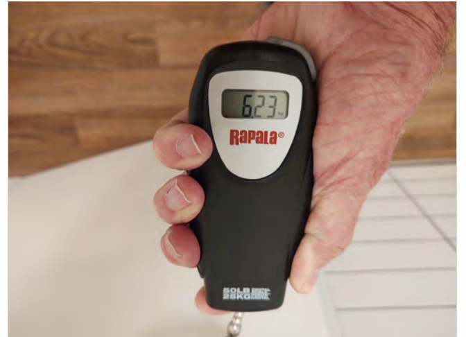
Photo FR8 – First Level Unisex Toilet Room – Measured door pull of 6.23 lbs.
