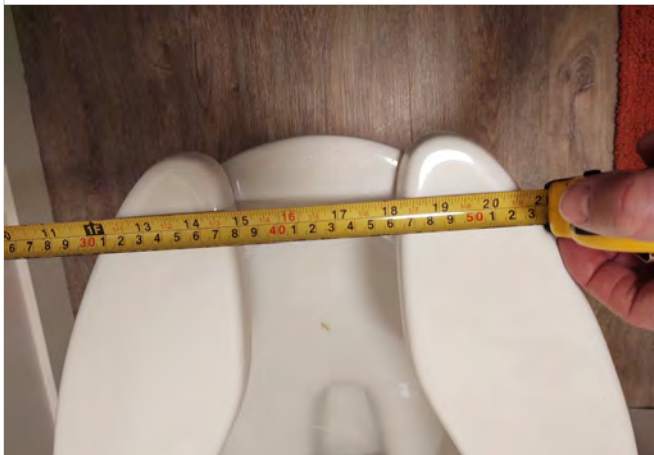
Photo FR23 – Dwelling Unit #212 - Measured dimension of 16 1/2" to centerline of water closet.
