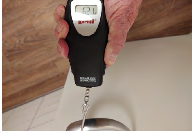
Photo FR10 – Third Level Unisex Toilet Room – Measured door pull of 6.21 lbs.
