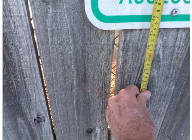
Photo B2 – Measured height to bottom of “Van Accessible” sign is 41 ½”
